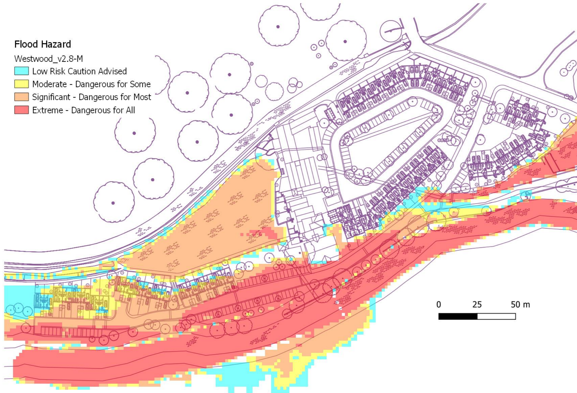
Figure B15: Post -development Scenario: Maximum Hazard for the 1 in 1000 year return period
