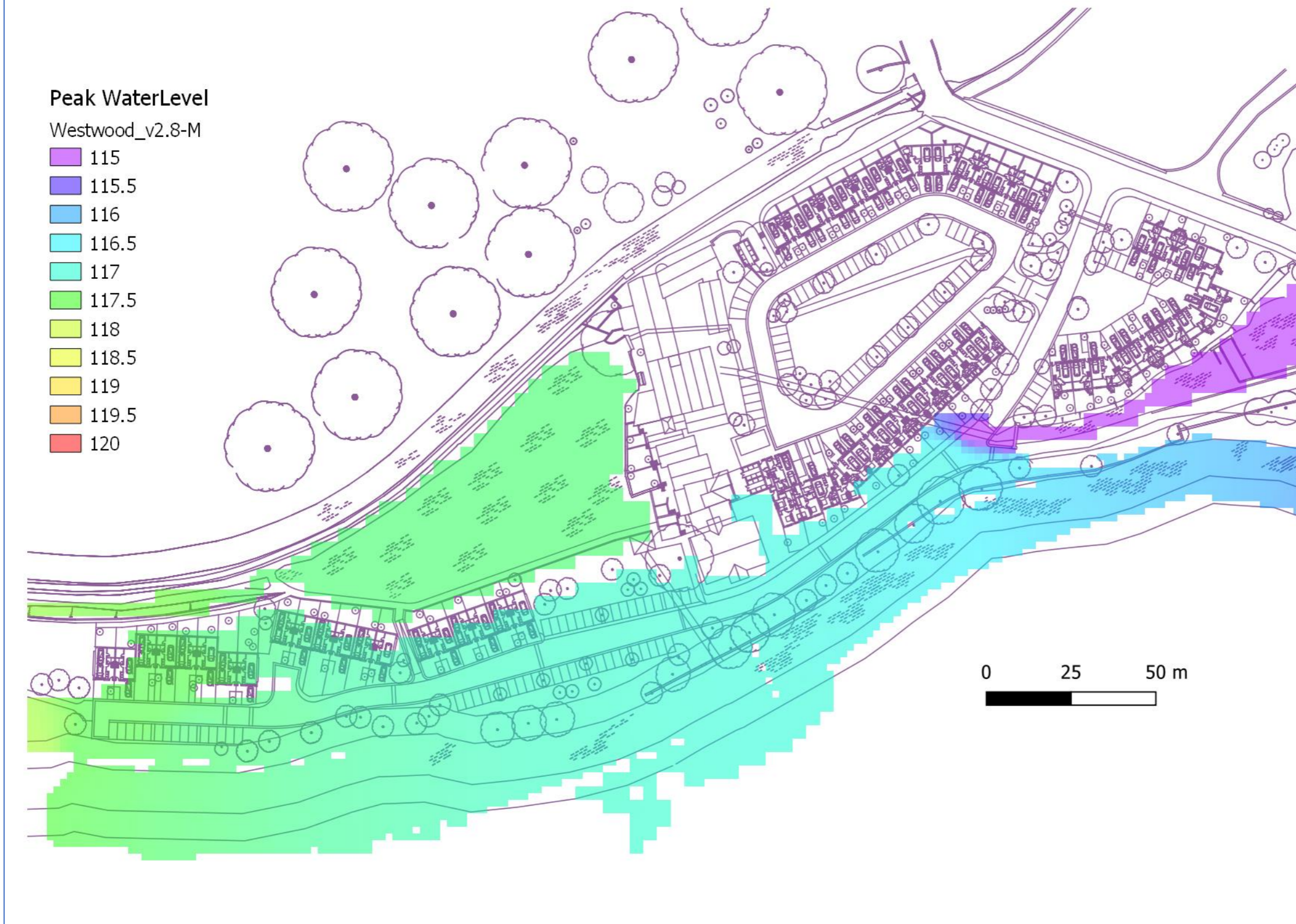
Figure B7: Post -development Scenario: Maximum Modelled Flood Level for the 1 in 100 year return period
